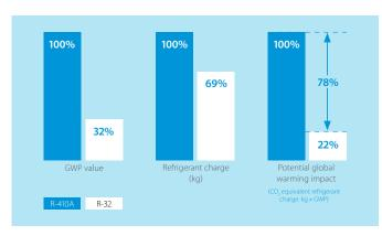
As a single component refrigerant, R-32 is also easier to recycle and reuse, which is another environmental bonus.
