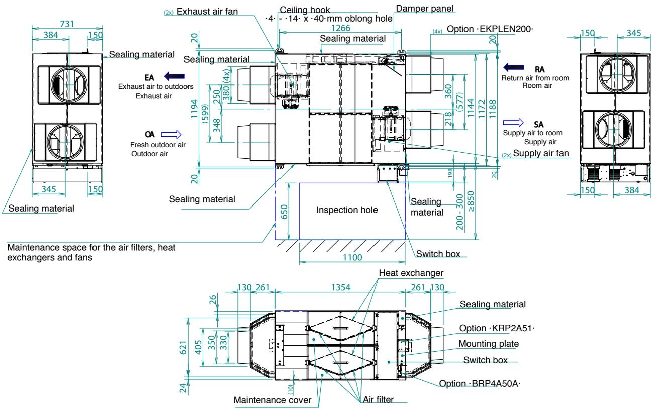
Maintenance space for the air filters, heat exchangers and fans
