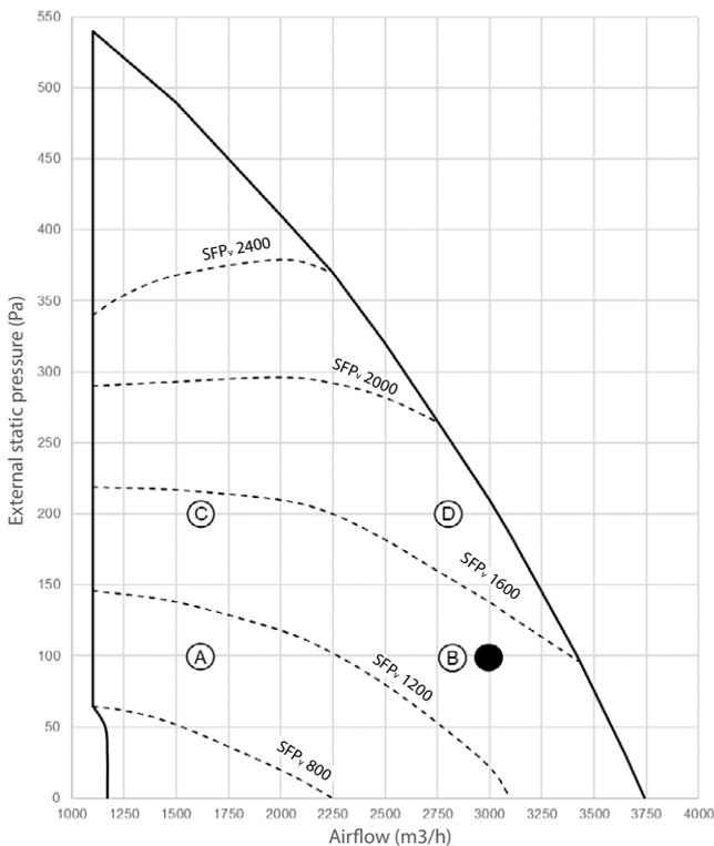
The diagram shows the available external pressure for the duct system given an airflow.
