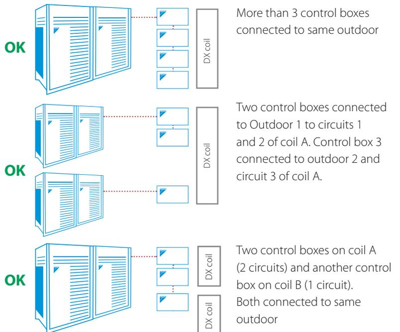
Multi application layout #2: Example for Z control with EKEQMCBA box and VRV indoor units
