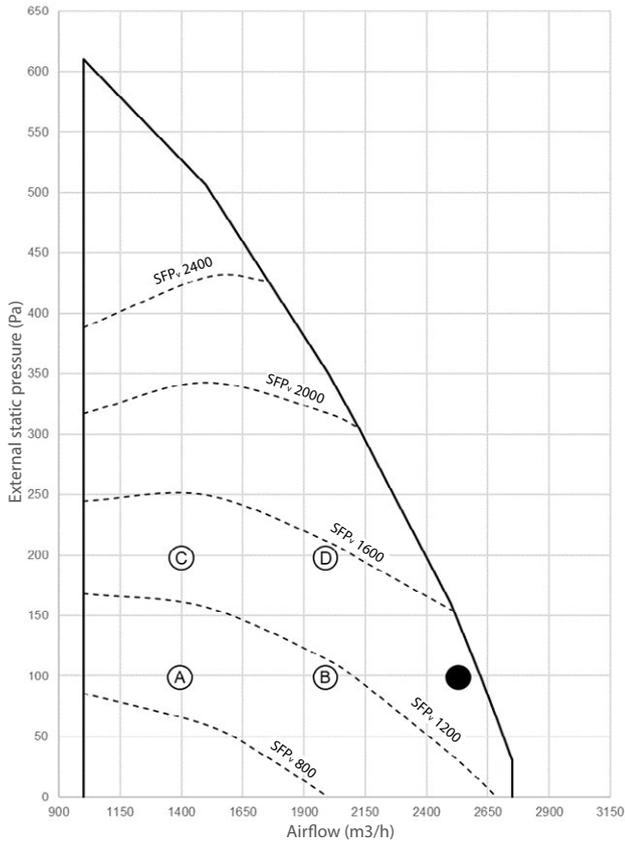
The diagram shows the available external pressure for the duct system given an airflow.
