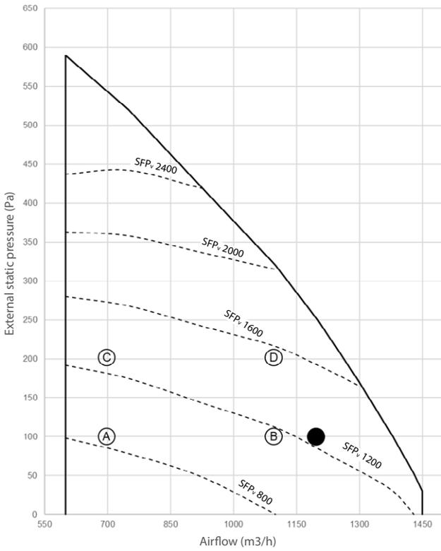
The diagram shows the available external pressure for the duct system given an airflow.
