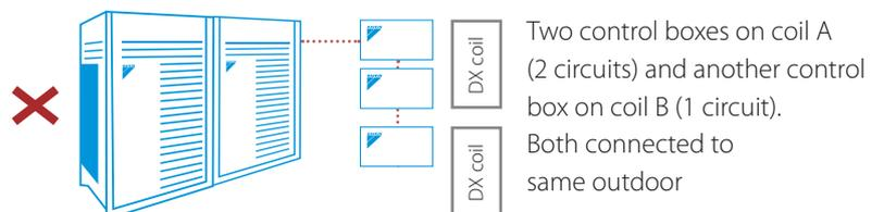
Pair application layout #2: Example for Y control with EKEQFCBA box
