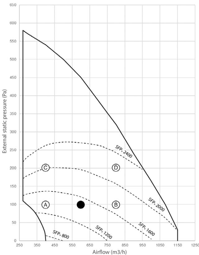
The diagram shows the available external pressure for the duct system given an airflow.
