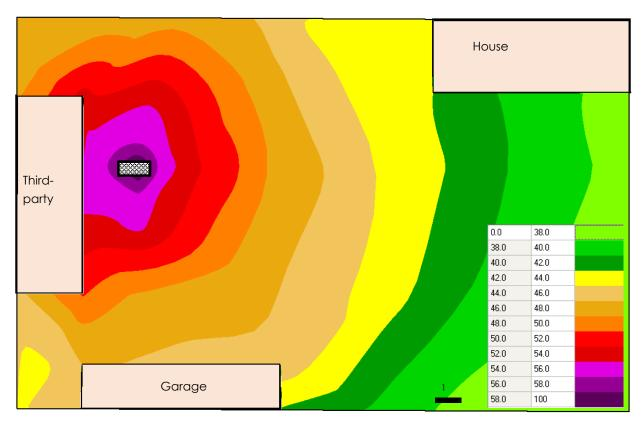
Maps of sound levels with the sound insulation enclosure:
