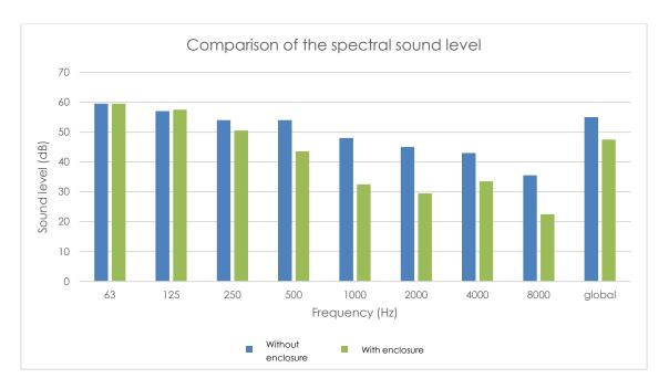
We notice a significant decrease in sound levels from 500 Hz onwards, and at all higher frequencies. The most significant decreases are located in the 1,000 and 2,000 Hz frequency bands.
